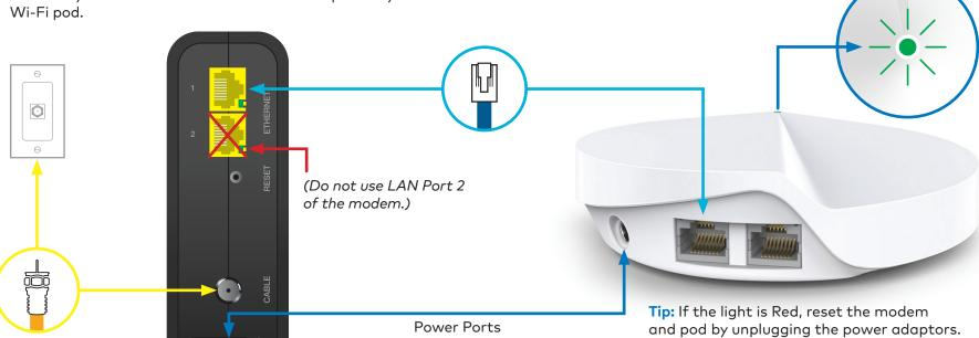
Attach the **Power Cord** to the **Power Port** on your modem, then plug the cord into a nearby power outlet.
